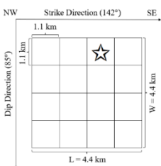
Fig. 1. Schematic illustration of the strong motion generation area of the August 18, 2020, Masbate, Philippines earthquake. The star represents the rupture starting point.
